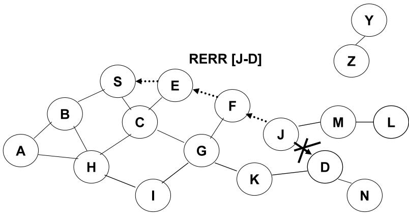
J sends a route error to S along route J-F-E-S when its attempt to forward the data packet S (with route SEFJD) on J-D fails
