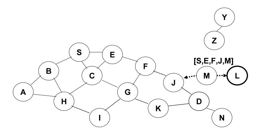
Node D does not forward RREQ, because node D is the intended target of the route discovery
